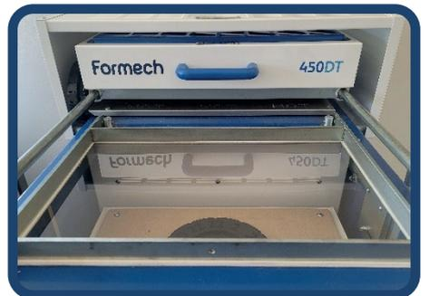
6. Place plastic sheet and send table down. All four heating zones are set up at 70% with a heating cycle of approximately 25-28 seconds. Material used: 0.5mm PETG
