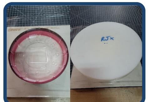
9. Place formed part into die cutter with clock face down, then place plastic board on top of formed part and die cutter.
