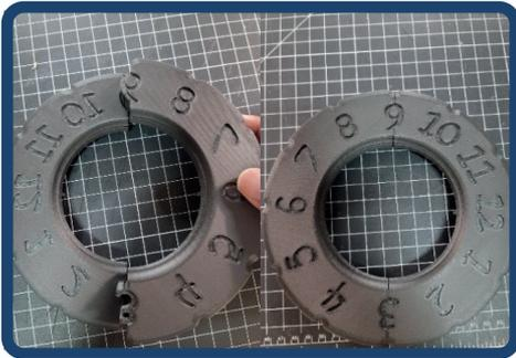
1. Connect the two outer portions of the clock face by sliding them together
